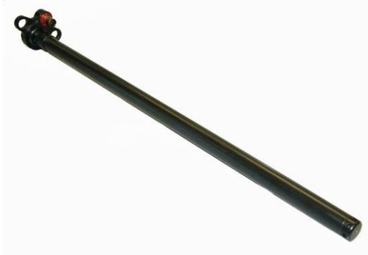
The output of the fluid level sensor is a voltage which changes in direct proportion to the level of fluid in the probe. There are no moving parts. The sensor operates by measuring the capacitance between the probe's two concentric tubes. Due to the difference in permittivity between air and the fluid being measured, the capacitance of the probe changes according to the ratio of air and fluid in the probe.
